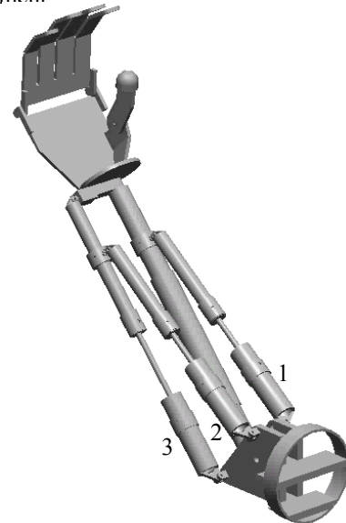
Figure 1. Schematics of a three degree of freedom parallel elbow. This elbow performs flexion, humeral rotation and pronosupination.
